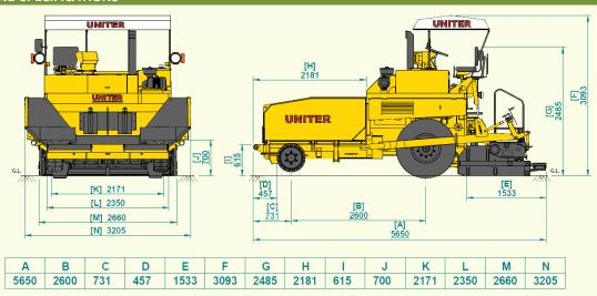
\* Dimension shown in above figure are measured in mm.
